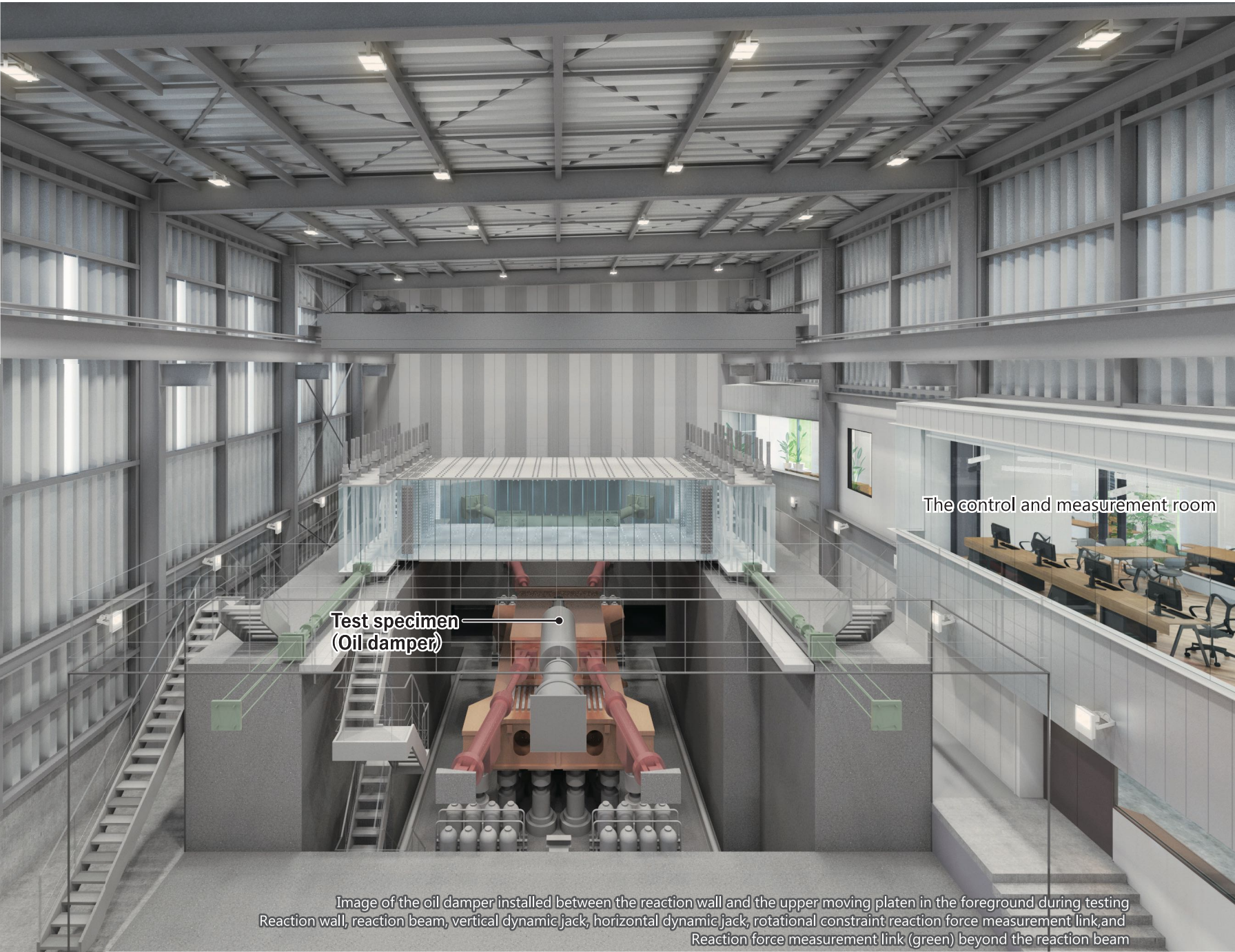
A control and measurement room for the testing machine is planned in close proximity, facing the full-scale seismic isolation testing machine. The test specimen under dynamic loading can be directly observed.
